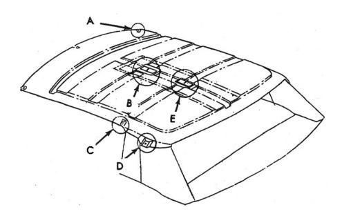
The illustration shows typical attachment points for a molded headliner. Details may vary from car to car but are easily seen. C is a screw through the coat hook area, D is a headliner retaining screw, A is the sun visor bracket screws, B and E are usually snap in fasteners that grip the headliner to the roof.
